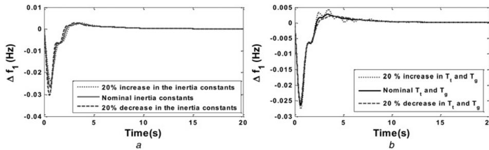
Fig. 9 Effect of power system parameters variation on the performance of the controllers tuned by the proposed MO method
