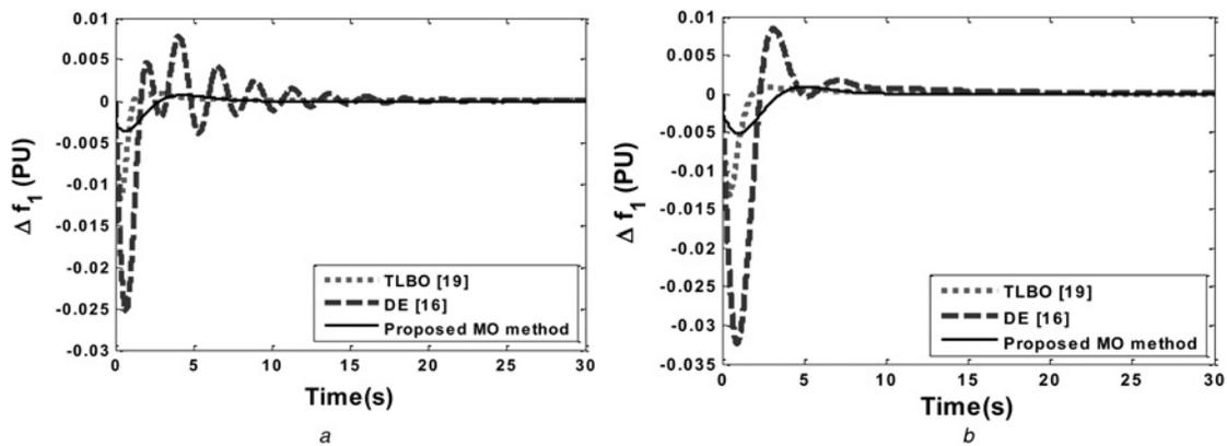
**Fig. 5** Change in the frequency of the first area for 0.01 pu increase in demand of area 1 in case of change in the topology of the system
