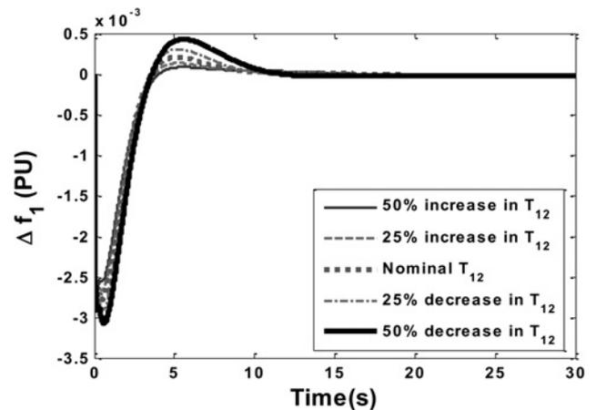
**Fig. 4** Performance of the controllers designed by the proposed MO method in case of a 0.01 pu increase in demand of area 1 with change in tie-line parameter
