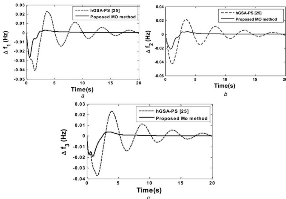
**Fig. 7** Frequency deviation of all areas in case of a 0.01 pu increase in demand of all areas
