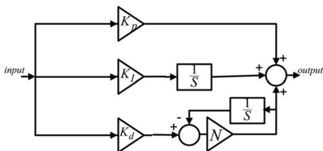
**Fig. 6** Schematic diagram of PIDF controller
