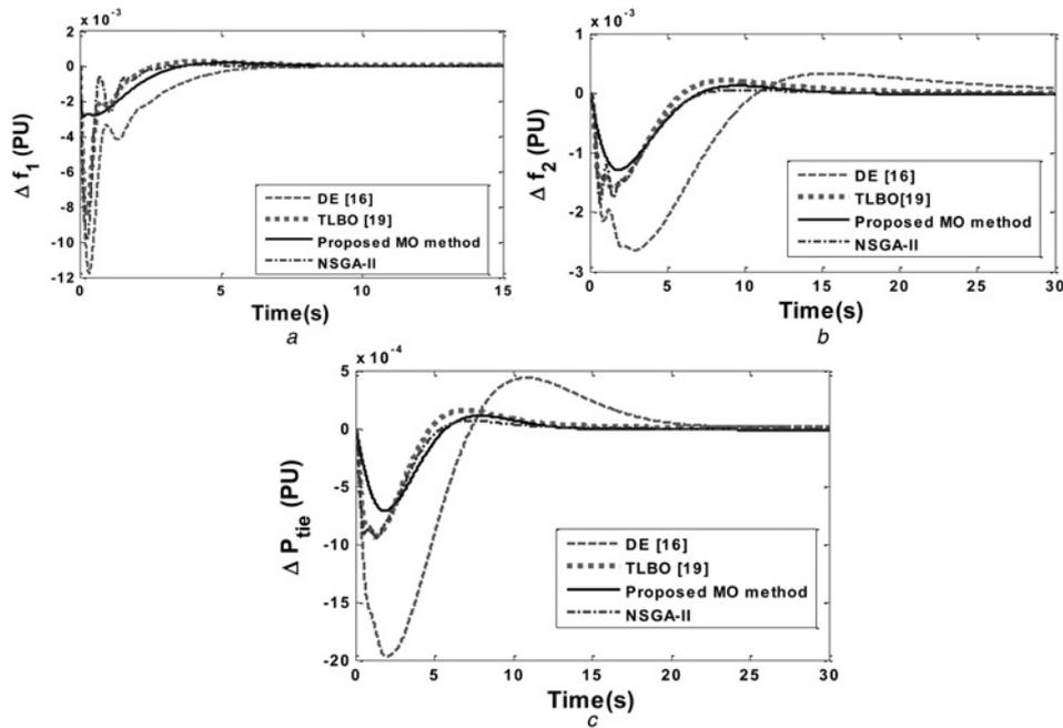
**Fig. 3** Performance of load frequency controllers in case of a 0.01 pu increase in demand of area 1
