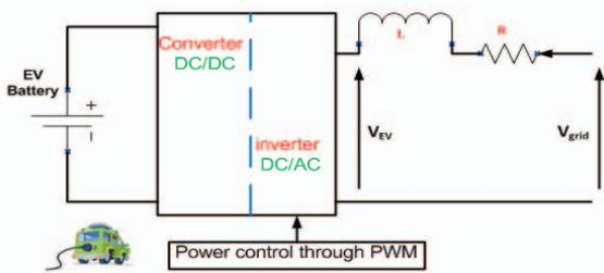
Fig1. Electric vehicle charger model [10].
