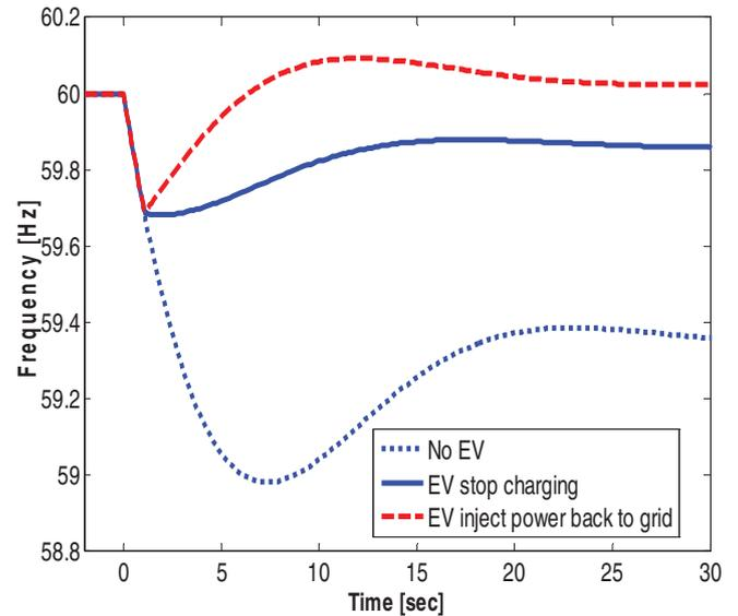
Fig.6 frequency response to the largest disturbance
