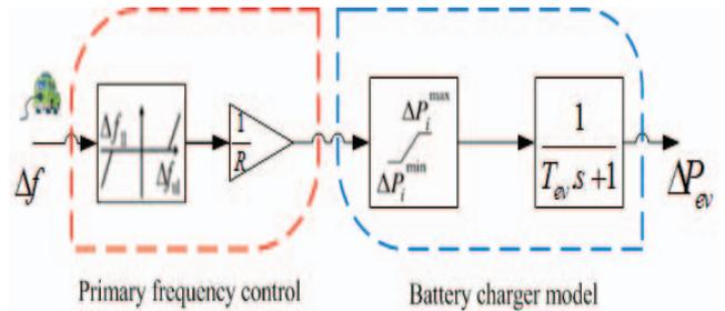
Fig.2. dynamic model of EV for primary frequency control
