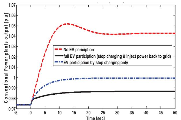
Fig.4 conventional power plant output
