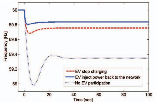
Fig.3 frequency response after disturbance
